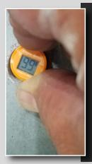
RH in the slab was reading 99%. This forced us to make the decision to use a moisture mitigating primer in order to keep on schedule and have no construction showdowns.
